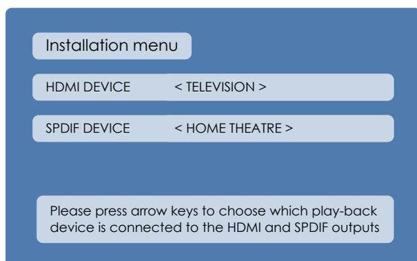
Figure 1: Logical and simple user settings in the installation menu that can be used to enable the set-top box to apply the right loudness levels.
