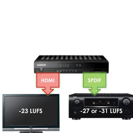
Figure B-1: TV connected to the HDMI, and the AVR connected to the S/PDIF, of a set-top box
