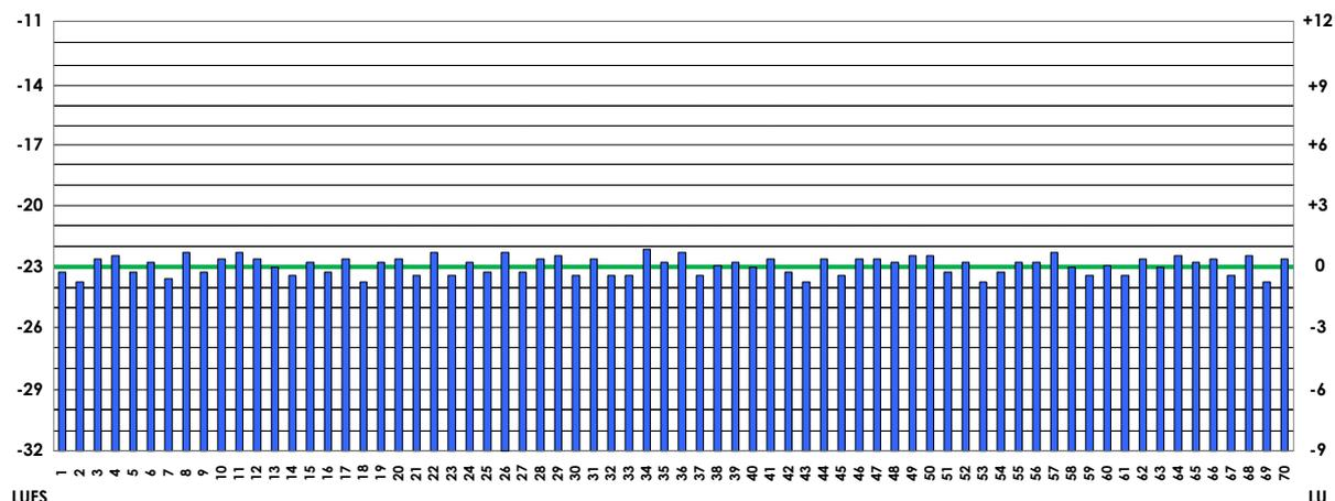
Figure A-1: Loudness levels at the output of a head-end. The services are listed on the x-axis. The left y-axis shows the absolute loudness level (in LUFS), and the right y-axis displays the loudness on the relative scale (in LU).
