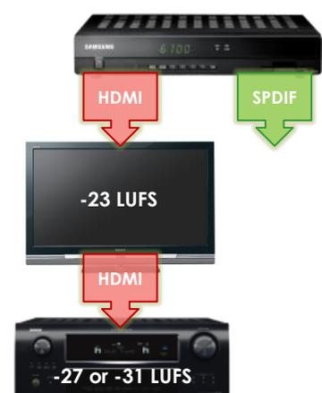
Figure B-3: TV connected to the HDMI of the set-top box while the AVR is connected to the HDMI of the TV, making use of its Audio Return Channel
