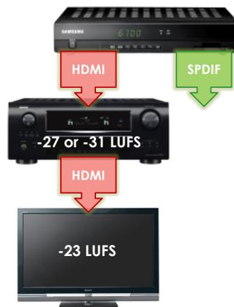
Figure B-2: AVR connected to the HDMI of the set-top box, TV connected to the HDMI of the AVR
