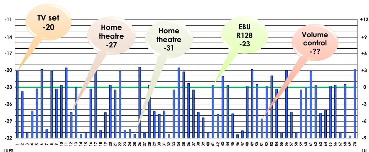
Figure A-2: The reproduced loudness level differs, depending on the equipment and the position of the volume control on the set-top box.
